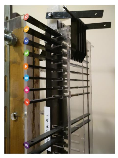
Figure 7: Photograph of constructed Memory address decoder
